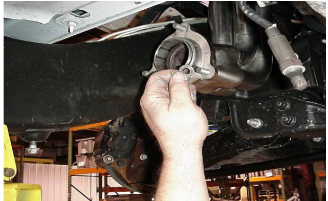
Install one spacer per stud to ensure proper connection with Y-pipe. (Both headers)
