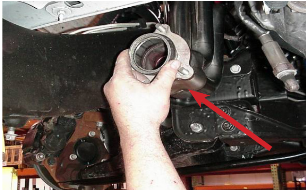
Install sintered donut gaskets before Y-pipe.
